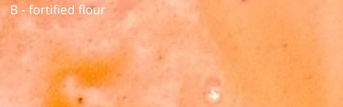
Photo: A picture of the zinc spot test developed by USAID AFFORD to help food producers and regulators quickly identify zinc in fortified foods. The dark pink and purple spots in the image on the right (B) indicate the presence of added zinc in fortified wheat flour. The image on the left (A) is of a non-fortified control sample. (Ashley Lamborn/USAID AFFORD)
