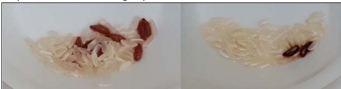
Figure 1: Fortified kernels in fortified rice will turn dark red/black, indicating the presence of iron.
